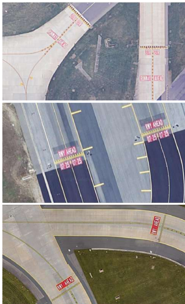
Figure 6. Example of 'RWY AHEAD' markings
