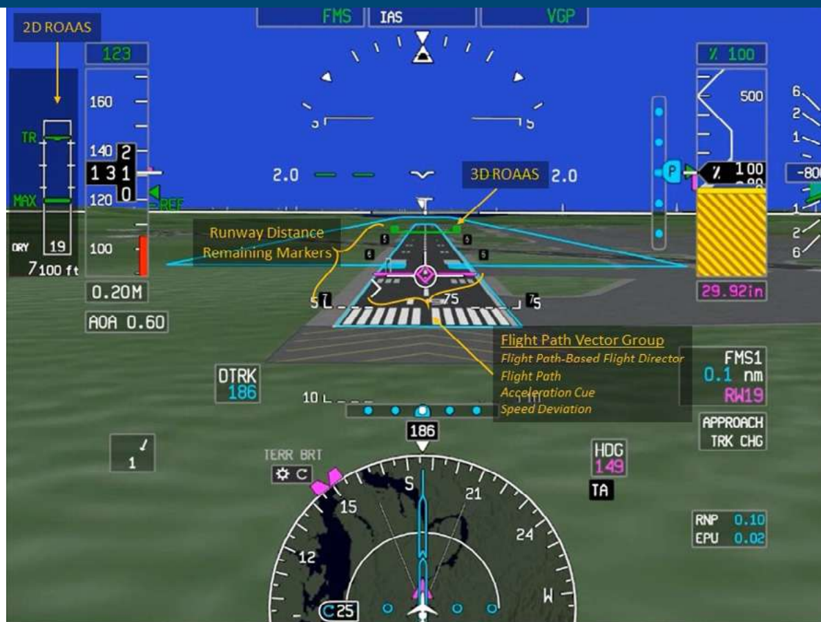
Figure 17. Example SVS with enhanced path and energy awareness
