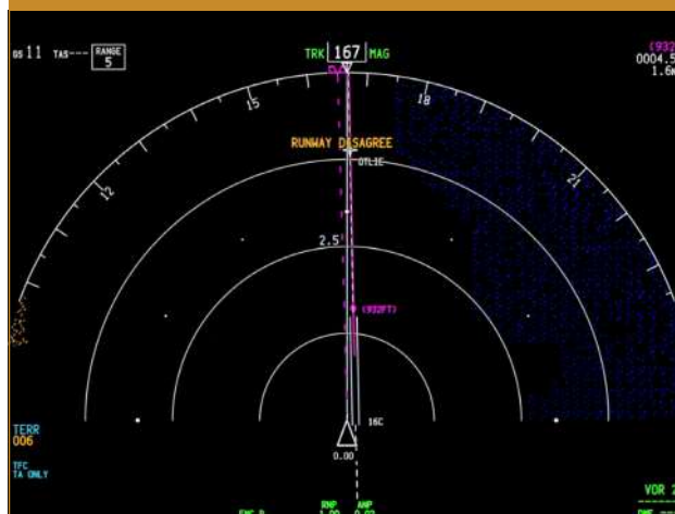
Figure 49. FMS runway disagree alert on the navigation display without airport map (© Boeing)
